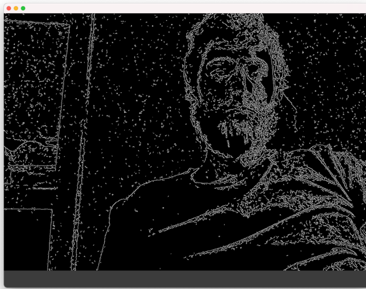
Figure 2 Canny Edge detection test on laptop using ofxCv
